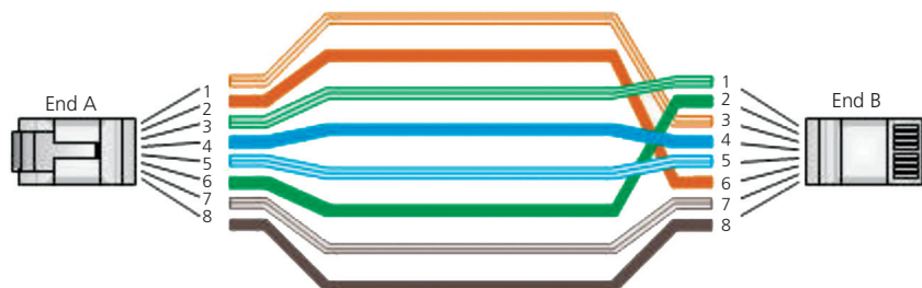
Figure C-3. Crossover wiring.
